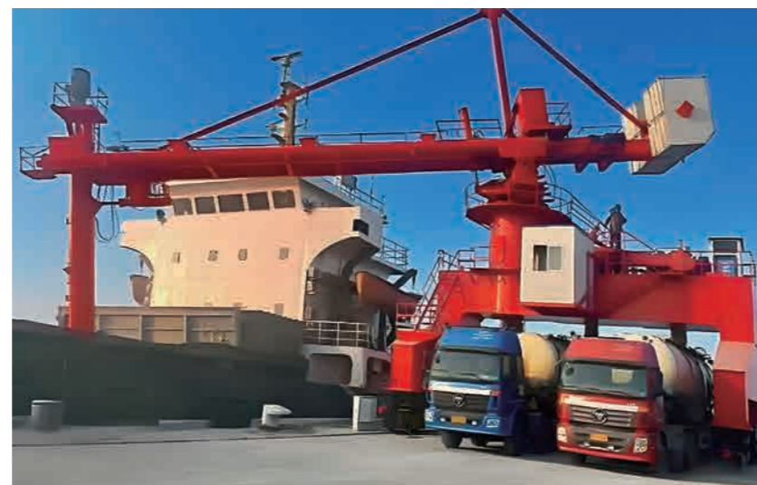
■ 连江冠海码头300吨移动卸船系统 Lianjiang Guanhai Wharf 300 tons Moved Unloading System
